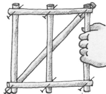
When testing the structure they should also be observing carefully where straws are beginning to bend and in what direction. This will help them understand how the load of the nails is being handled by the structure.
